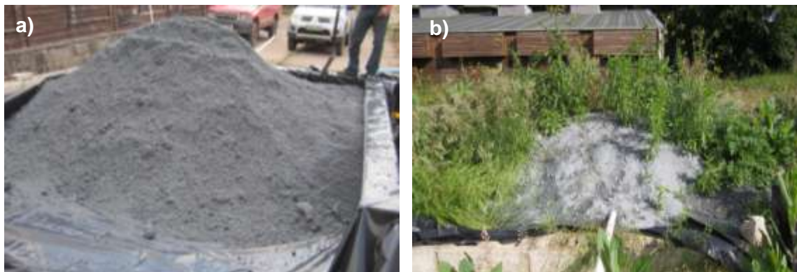
Figure 3. Paper sludge heaps at the start (a) and end (b) of the storage period
