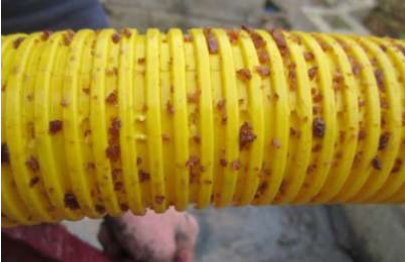
Figure 0-12. Salt crystals on the pipework within PLA Heap 3
