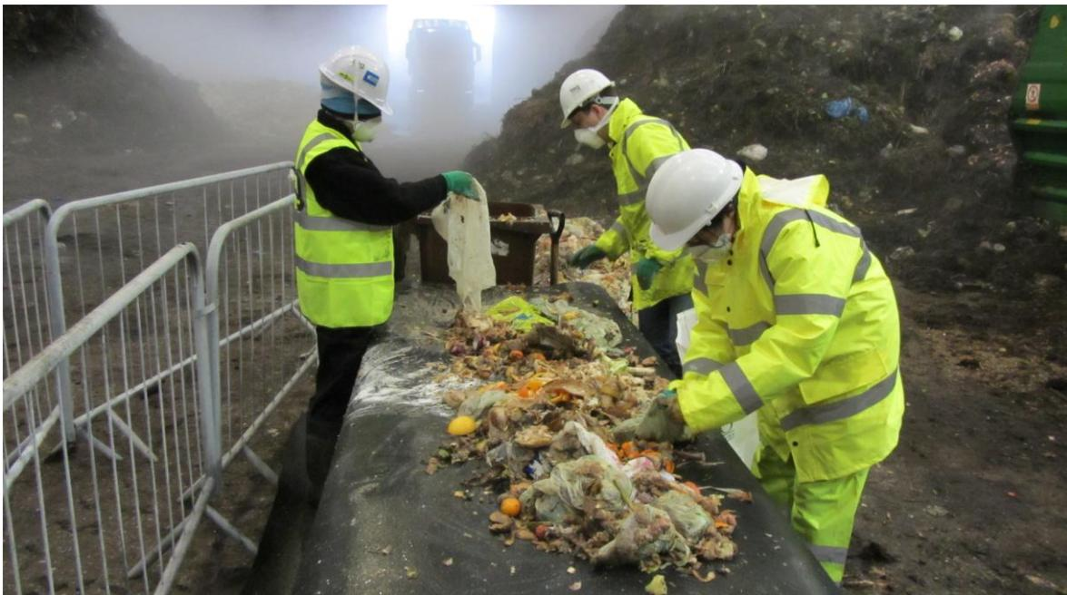
*AfOR, TEG Environmental and Novamont staff sorting non-compostable and compostable materials from a sample of bagged food wastes.*
